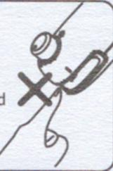
Battery Installation (2\*AA alkaline batteries) 电池安装 (AA 五号碱性电池\*2个)
